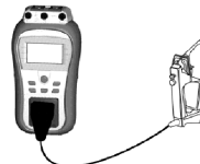
Test circuits for touch leakage current measurement
